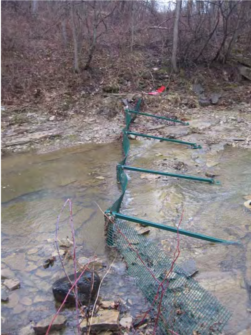
View showing degree of bowing on bottom screen.
