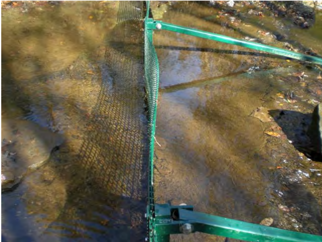
Photo 3: Downstream (1-inch grid opening) screen deflection
