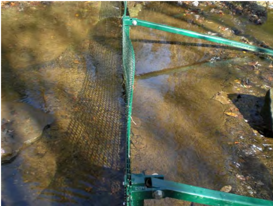
Photo 3: Downstream (1-inch grid opening) screen deflection
