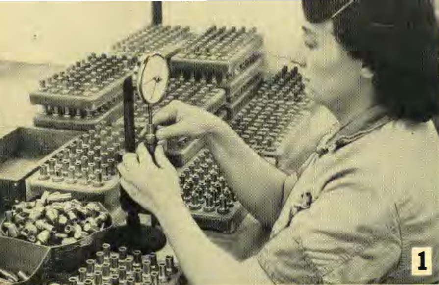
Anna Swartzlander gauges a fuze head as one of the many inspection operations in fuze assembly. Inspections such as these assure us that our "matches" will "burn".
