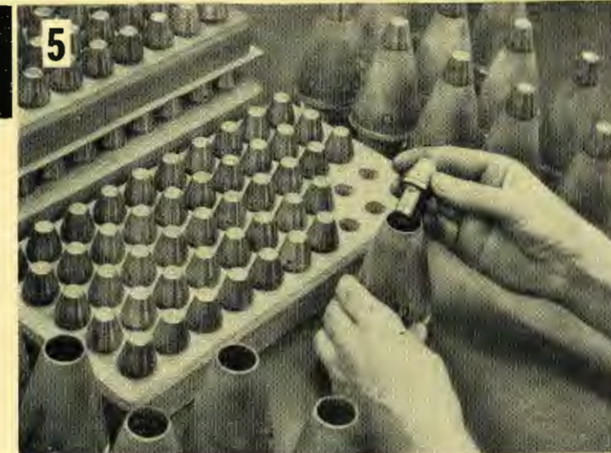
Loaded fuze heads are attached to the fuze body after the ogive or windshield has been slipped into position.
