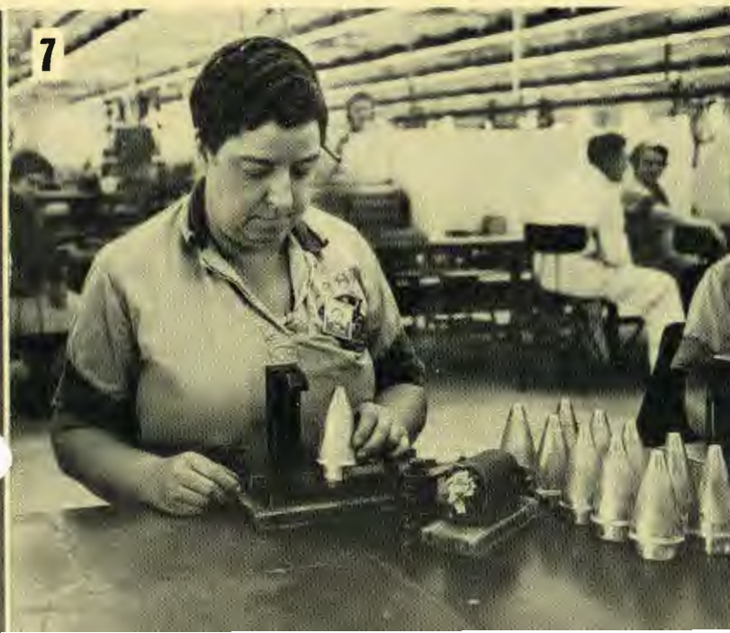
After the fuze head is inserted its threads are destroyed in the staking machine.
