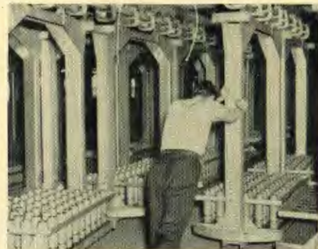
Shells are allowed to dry on mono-rail dollies.
