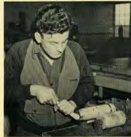
Threads are cleaned of all foreign matter.
