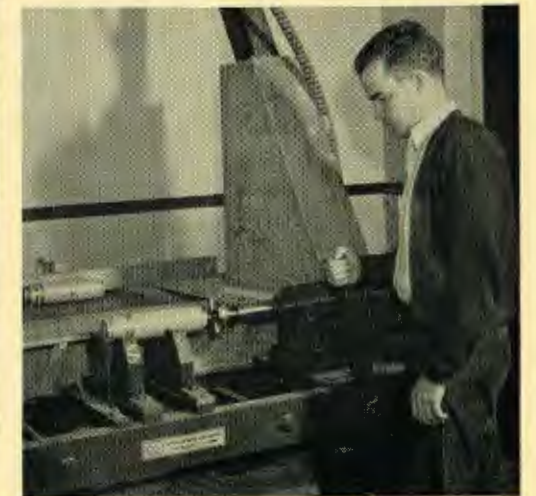
A booster cavity is drilled in hardened T. N. T.
