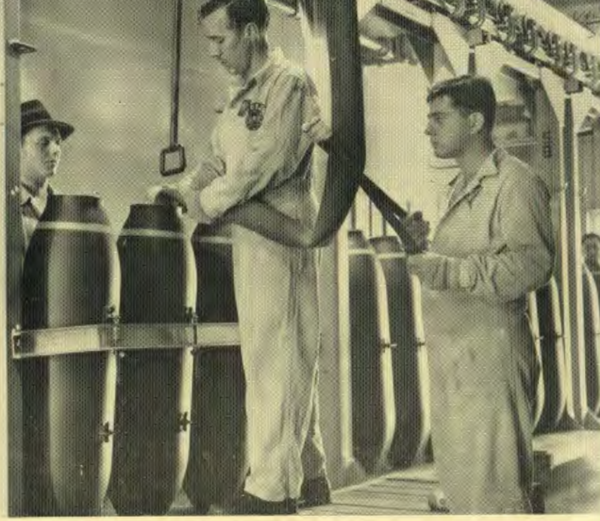
BOMBS ARE NEXT FILLED WITH amatol. Left to right are Joseph Polack, bay leader; Ernest Tedrich, hose operator; Mike Frasca, who controls flow of explosive.
