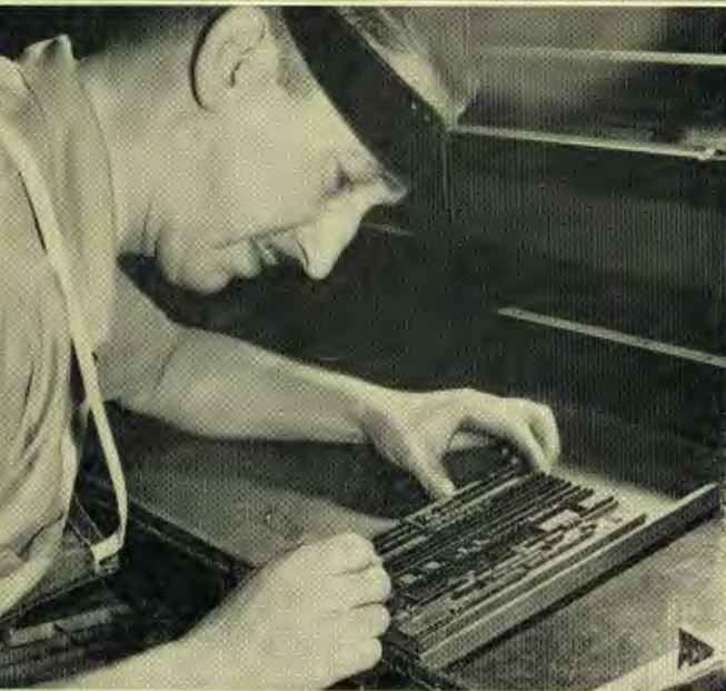
Compositor pictured at left, is William Ebby, setting type that will be used to make rubber plate.
