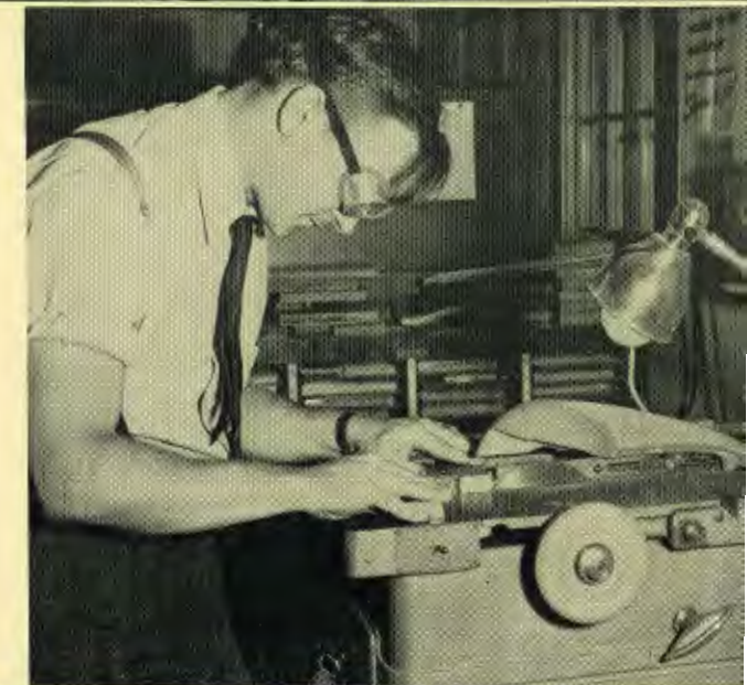
Using safety glasses at the power saw is Tommy Jones. The saw is used to "true up" engravings or "slugs" of type.
