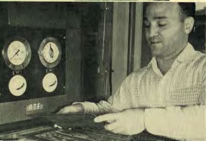
The rubber plate is peeled from the bakelite mat after it has been heat "cured" for ten minutes in the Precision machine.
