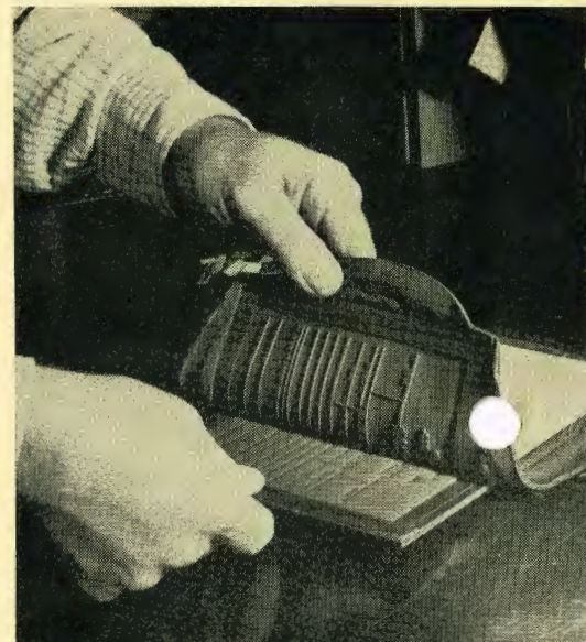
The rubber plate is peeled from the bakelite mat after it has been heat "cured" for ten minutes in the Precision machine.
