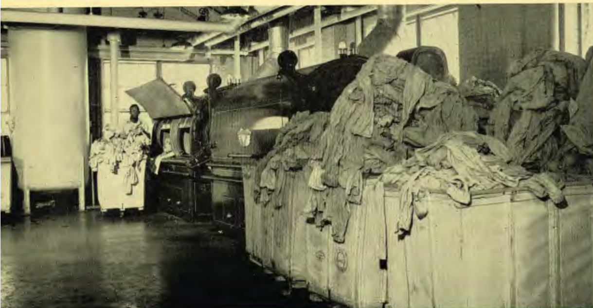
After the coveralls are removed from the "washer", pictured at extreme right, they are placed in one of the two centrifugal driers.
