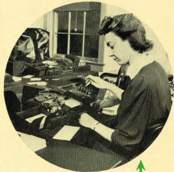
Miss Helen M. Ladrach takes the information found on the daily time cards and, with this duplicating key punch, prepares cards for use in the alphabetic accounting machine.
