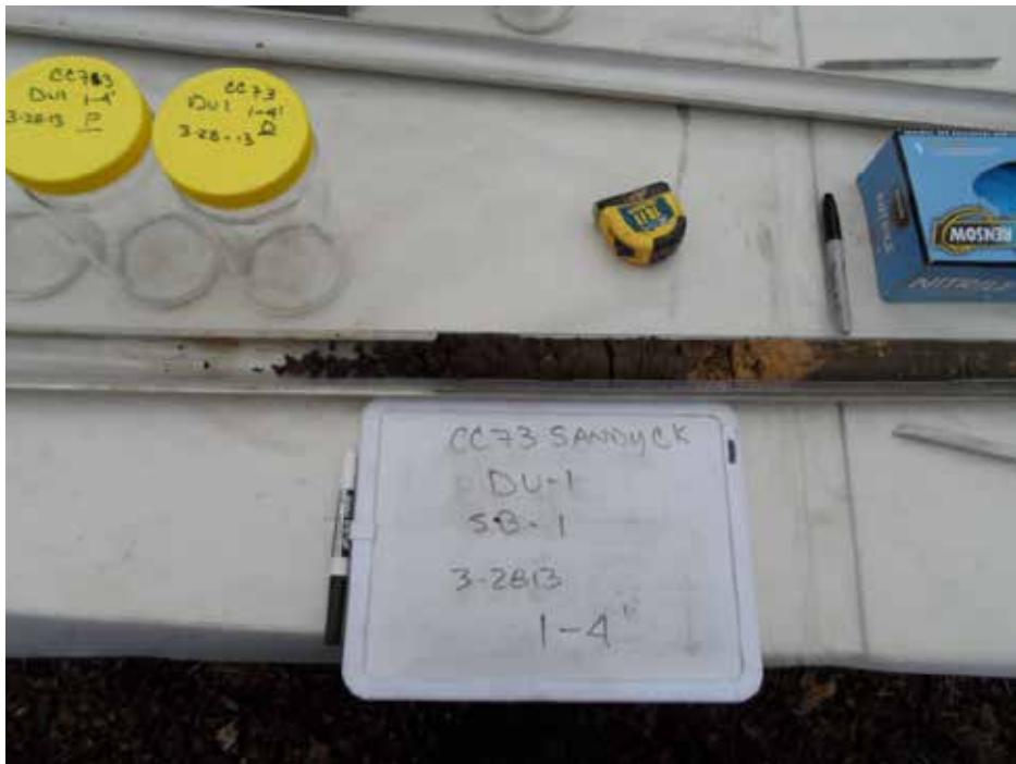
Soil classification, logging, and sampling at DU01 SB01, located at the Sand Creek Coal Tipple (March 2013).
