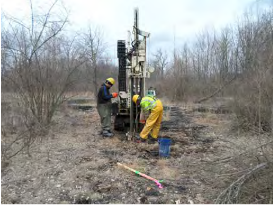
Soil boring utilizing a GeoProbe at North Line Road Coal Tipple (March of 2013).
