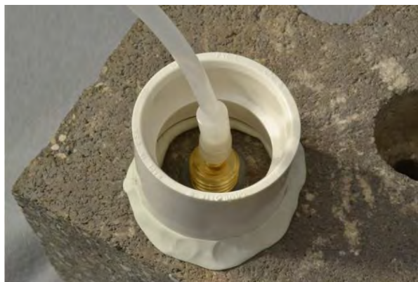
Figure 6. Water dam used for leak detection
