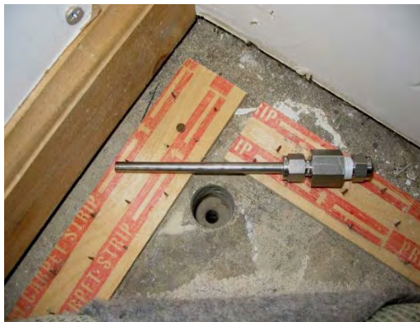
Figure 1: Assembled sub-slab port ready for installation
