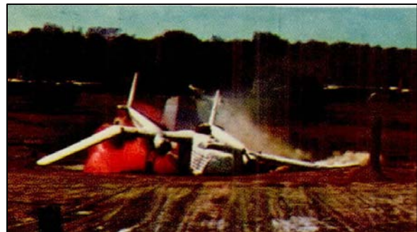
Photograph 4. C-82 1-Second After Initial Impact with Crash Barrier Airplane Used at NACA Test Area (NACA 1953, Figure 41b)
