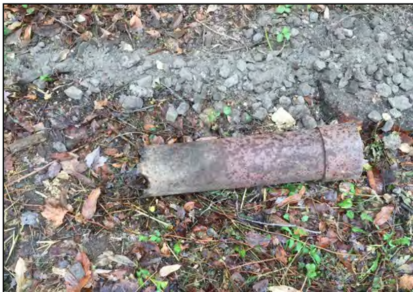
Blocked casing removed from Well 66.
