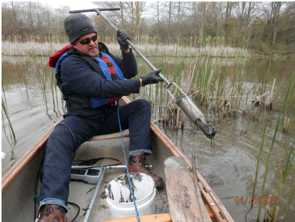
11. Photograph of hand corer used to collect sediment sample from sampling location 079SD-112.
