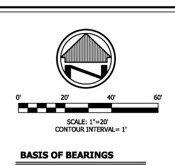
THE BASIS OF BEARINGS FOR THIS SURVEY IS GRID NORTH OF THE OHIO STATE PLANE COORDINATE SYSTEM, NORTH ZONE, NAD88 (2011).
